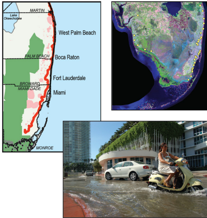
Figure 17.8. Sea level rise presents major challenges to South Florida’s existing coastal water management system due to a combination of increasingly urbanized areas, aging flood control facilities, flat topography, and porous limestone aquifers. For instance, South Florida’s freshwater well field protection areas (left map: pink areas) lie close to the current interface between saltwater and freshwater (red line), which will shift inland with rising sea level, affecting water managers’ ability to draw drinking water from current resources. Coastal water control structures (right map: yellow circles) that were originally built about 60 years ago at the ends of drainage canals to keep saltwater out and to provide flood protection to urbanized areas along the coast are now threatened by sea level rise. Even today, residents in some areas such as Miami Beach are experiencing seawater flooding their streets (lower photo). (Maps from The South Florida Water Management District. 36 Photo credit: Luis Espinoza, Miami-Dade County Department of Regulatory and Economic Resources).
